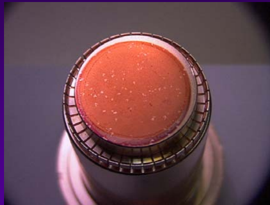
Photocathode after 170 working hours in the DC gun @ 8 MV/m and 7nC/pulse 8 ns, 10 Hz, P \leq 5 \times 10^{-10} mbar QE_{start} = 16.4\% ; QE_{end} = 4.2\%
