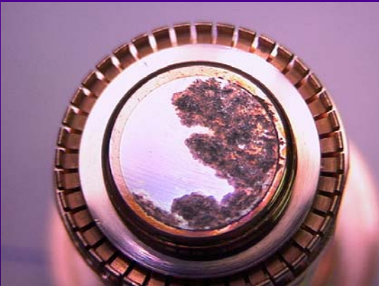
Cu photocathode destroyed at 85 MV/m during conditioning process
