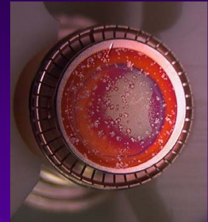
Photocathode after 148 working hours in the RF gun @ 105 MV/m, 180 nC in 24 pulses, 10 ps FWHM Rep. rate = 5 Hz, P \sim 2 \times 10^{-9} mbar QE_{start} = 11.4\% ; QE_{end} = 2.2\%
